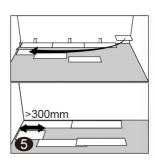
6. Second row, second plank: Click the long side of the plank into the previous row and place it tight to the short end of the previous plank at an angle of 25-30°. Drop the plank and gently tap on the end with a rubber mallet so it firmly locks into the previous plank until both are at the same height. Make sure both planks are perfectly aligned.
